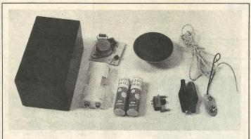
This photo shows all of the required components prior to assembly. Although utility boxes are available in many different sizes, this one neatly holds all the parts, yet it is compact enough to fit in your toolbox.
