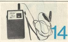
It's even cheaper to convert an old transistor radio into a buzz-box since it already has a speaker, an on-off switch and a battery snap. The ear-piece plug assembly can be converted to accommodate the alligator clips by cutting off the ear piece and installing the clips. If you want, you can even drill a hole in the module board and mount it in the case where the radio board was mounted.
