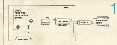
This is the basic wiring diagram for the oscillator unit. As you can see, it is quite simple and all you need for assembly is a soldering gun and a small amount of solder. The A, B, and C terminals shown on the diagram are actually printed on the code practice oscillator board so it makes the operation almost foolproof.
