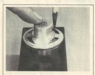
Position the speaker on top of the box as shown here, then draw a pencil line around the circumference. Next, drill several holes within the outline. These holes let the speaker's sound out of the box so you can readily hear it. Just a few random holes will suffice, or you can drill a professional-looking pattern. But remember, if you drill a bunch of holes, drill slowly and with light pressure because the case is made of plastic.
