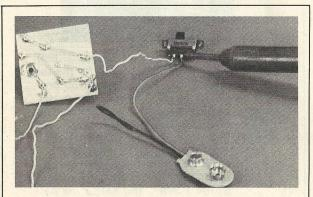
Solder the wire from the A terminal on the module to one side of the switch. Next, solder the red wire from the battery snap to the other switch terminal as shown here. Caution: It is very important to have the red wire from the battery snap connected to the switch. This insures the correct polarity as shown in the wiring diagram.
