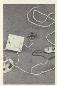
Following the wiring diagram, connect the B wire from the module to one side of the speaker. Take the test lead wires and solder one of them to the C wire from the module. Now, solder them to the other side of the speaker as shown. Attach the other test lead wire to the black lead from the battery snap and solder; cover this junction with a small piece of electrical tape. The knots tied in the test lead wires prevent them from being pulled out of the case.
