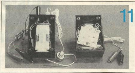
There are alternative ways to build one of these units as long as the oscillator is wired into the system. The unit on the left uses an ear plug and phone jack instead of a speaker and a switch; the alligator clips connect to the phone jack wires. The phone jack acts like a switch; when it's unplugged, the unit is off. But the amount you save on the speaker and switch is about the same you will spend for the ear plug and phone jack, so this one is priced about the same as the previous one.
