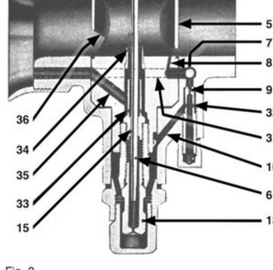
Fig. 3 -Diagrammatic section of Carburetter showing only the lower half of the throttle chamber with the throttle a little open - and the internal primary air passages to the main jet and pilot system
